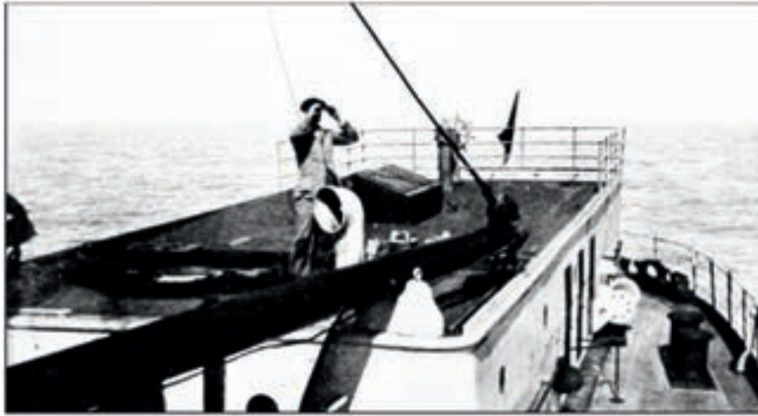
The look-out man is disguised as a member of the Mercantile Marine and the ship's wheel, sky-light and deck-house are of a superficial nature, concealing a 4-inch gun and two 12-pounders
